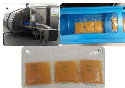
**Figure 1:** Representation of the high-pressure assisted extraction. Showing the high pressure equipment (A) used, samples before (B) and after (C) the extraction process.
