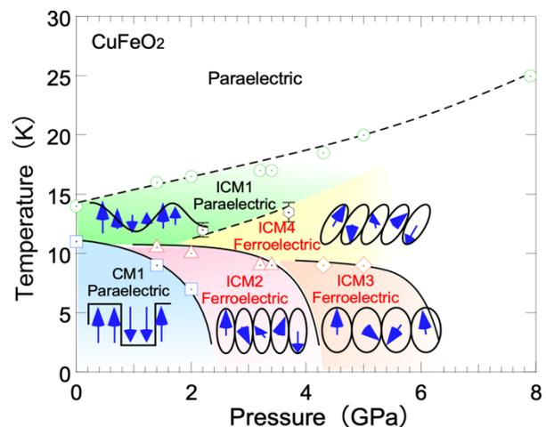
Figure 1. Pressure versus temperature phase diagram of multiferroic delafossite  $\text{CuFeO}_2$ . [5]
