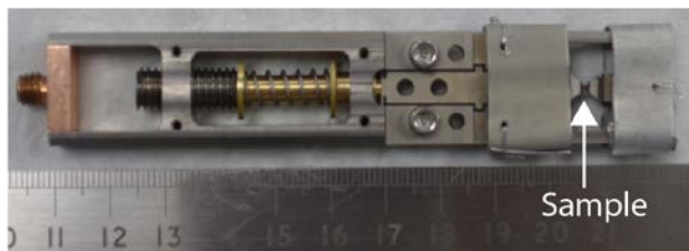
Figure 1. The overall appearance of the uniaxial pressure device for neutron diffraction experiments. The shown configuration of the device is for applying a compressive load. Force is applied to a moving part of the sample holder, whose motion is constrained by flexures to be longitudinal with respect to the sample. This protects the sample from inadvertent transverse or twisting forces. Each end of the sample is secured with epoxy between 2 Ti sample plates.
