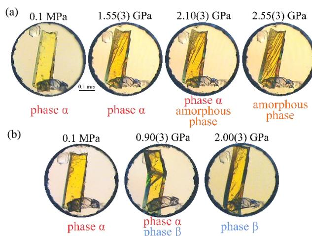
Figure 1. The sample C5-PPB single crystal (a) first compressed rapidly to 1.5 GPa, when the wrinkles mark the onset of amorphization, and then (b) after releasing pressure it was compressed again slowly to 0.9 GPa, where the transition to phase  $\beta$  starts and transition fronts travel through the sample, till it all transforms to the end.
