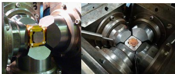
Figure 1. The SSA mounted in the first-stage anvils of MAX-80 installed in BL NE5C, KEK-AR. The conventional assembly (left) requires more than 1 hour, whereas the new assembly (right) allows a single user to finish setting within 10 min.
