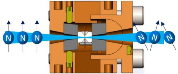
Figure 2. Section cut of a CuBe moissanite anvil cell used in the experiments, illustrating how the polarized neutron beam easily accesses the sample space through the optical aperture.
