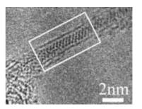
Figure 1. HRTEM image of DWCNTs filled with 1D nanocrystalline CdSe
