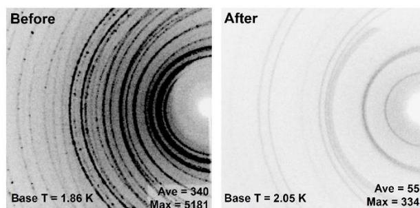
Figure 1. Two frames (20 s exposure time, 0.5° rotation) with the same colour scaling before and after improvements. Insets show the base temperature achievable with the respective setups and the average and maximum intensity on the image.
