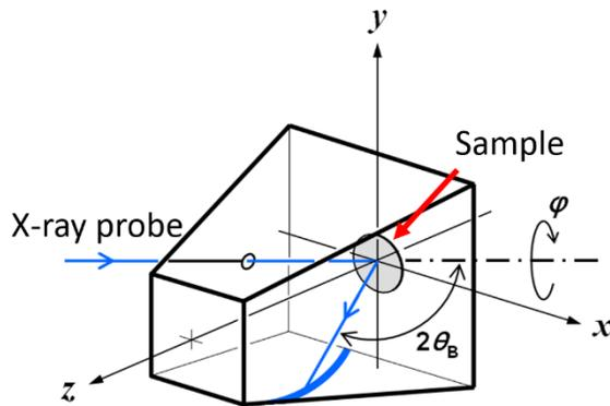
Figure 1: A diagram showing the layout of our x-ray probe, sample and image plates, which lie on the trapezium shaped sides of the box.
