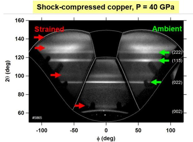
Figure 2: X-ray diffraction data recorded from shock-compressed copper, with three trapezium shaped image plates mapped onto a  $2\theta$ ,  $\phi$  plot. Both the narrow Debye-Scherrer rings from the ambient material, and the broader rings from the compressed material are recorded on the image plates.
