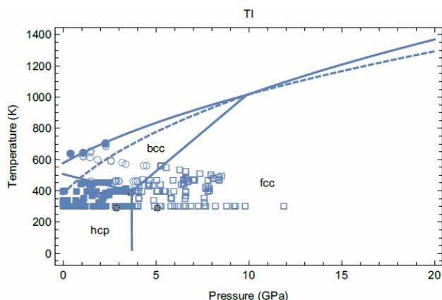
*Figure 1.* The phase diagram of thallium that combines experimental data points and *ab initio* phase boundaries
