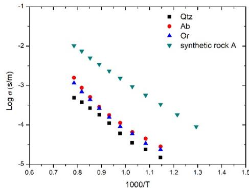
Fig 1. Electrical conductivity of three single phase minerals--Quartz, Albite and Orthoclase, as well as the synthetic rock A
